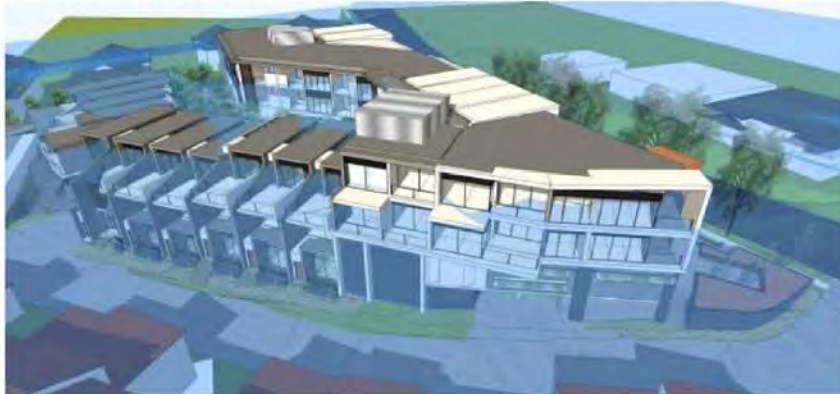
HEIGHT PERSPECTIVE 2 (IMAGE ABOVE DISPLAYING BUILDING ELEMENTS OVER THE 9m HEIGHT LIMIT RELATIVE TO NATURAL GROUND LINE)
