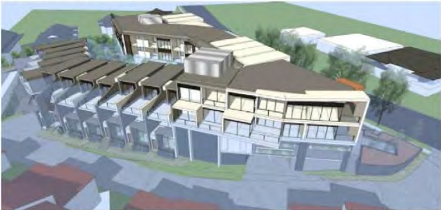
HEIGHT PERSPECTIVE 2 IMAGE ABOVE DISPLAYING BUILDING ELEMENTS OVER THE 9m HEIGHT LIMIT RELATIVE TO BASEMENT LEVEL
