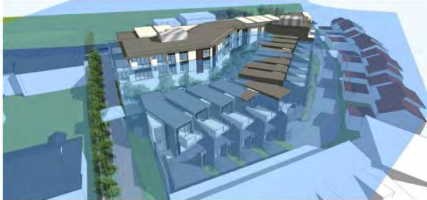
HEIGHT PERSPECTIVE 1 (IMAGE ABOVE DISPLAYING BUILDING ELEMENTS OVER THE 9m HEIGHT LIMIT RELATIVE TO NATURAL GROUND LINE)
